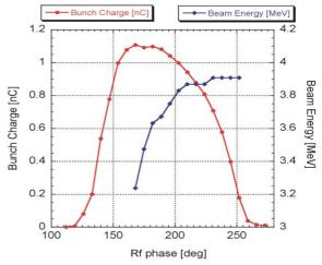
Fig. 2 Bunch charge and beam energy dependences by changing Rf phase
