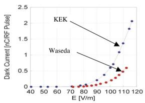
Fig. 1 Dark current measured under the beam test with the high gradient acceleration fields
