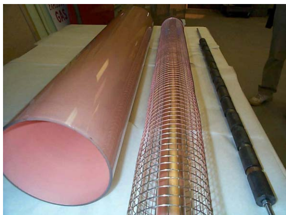
Figure 5. Anode screen shown with Cu cathode, magnet string and coated glass tube.
