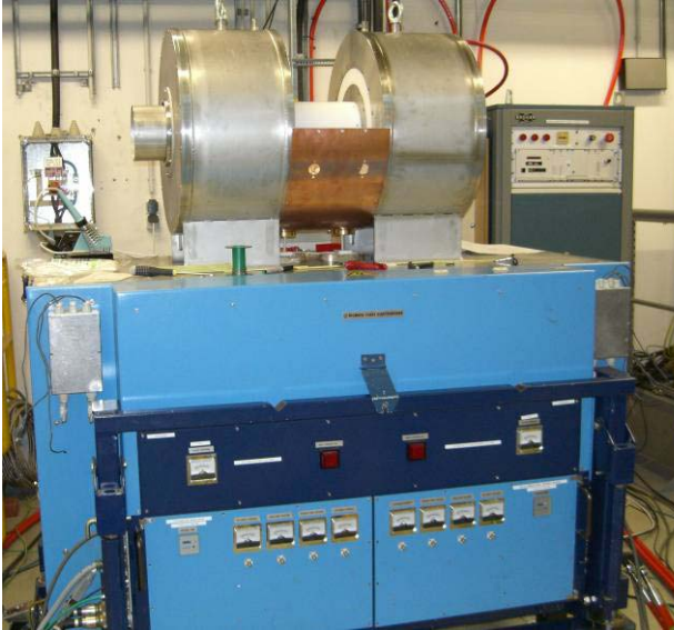
Figure 2: Accelerating cavity installed on top of the former COSY tube amplifier.
