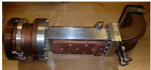
Figure 7 : Assembly of microwave line parts on the high voltage side (from left to right VIS plasma chamber, matching transformer and the water-cooled bend).
