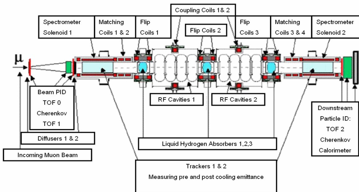
Figure 1: MICE Cooling Channel
