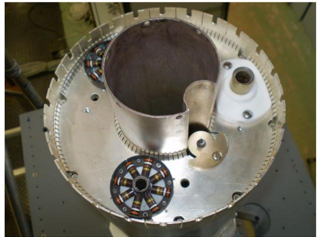
Figure 6: Input Cavity Tuning Annulus after Silver Plating and replacement of Fingerstock
