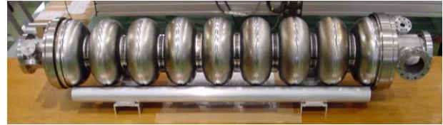
Figure 1: A TESLA-like STF-Baseline 9-cell cavity, [2].
