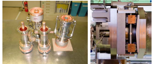
Figure 2: Left is two pairs of cold and warm couplers, [3]. Right is a frequency tuner system, [4].
