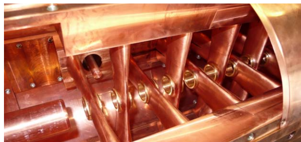
Figure 8: Photograph of the r.t. copper model to validate electrodynamic simulations.
