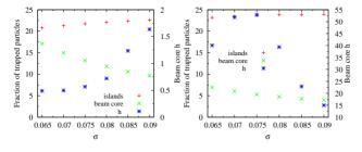
Figure 4: Fraction of trapped particles as a function of the initial sigma. Two types of tune curves are used: 1-1 (left) and 2-3 (right). The value of the factor h for the beam core is also given.
