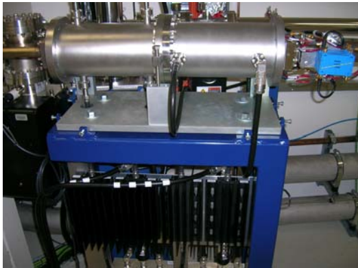
Figure 7: The kickers are seen along with the attenuators. Behind the attenuators are the low-pass filters and splitter for each channel (x and y).
