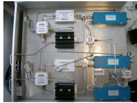
Figure 4: The physical layout of the analogue front-end produced by the Australian Synchrotron. Both x and y channels visible.
