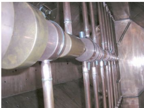
Figure 9: Accelerating structure after final tuning (at the left above – RF-input).
