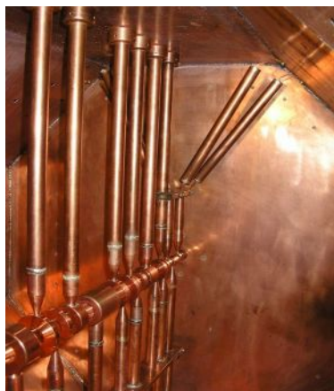
Figure 4. The end resonant tuning element and additional stems on the entrance end accelerating structure.
