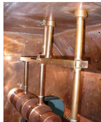
Figure 3: The end resonant tuning element on the exit end accelerating structure.
