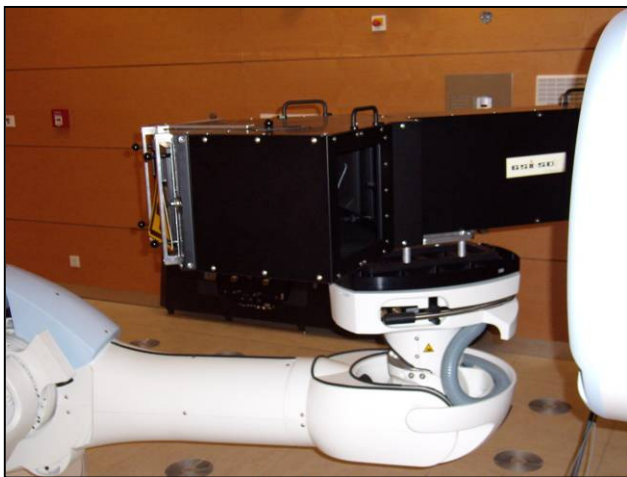
Figure 5: Isocenter diagnostics mounted on patient robot.
