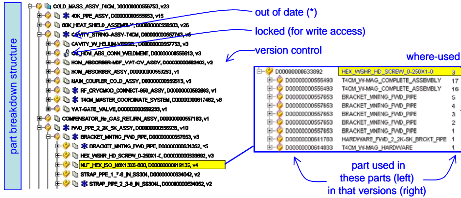
Figure 4: Data management controls the hierarchical structure of design models (left) and keeps track of part usage (right).
