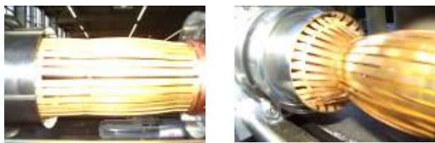
Figure 5: Shape of the RF fingers at critical span for nominal and large angle
