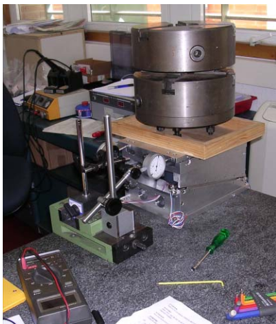
Figure 7: Test of horizontal movement with dummy mass.
