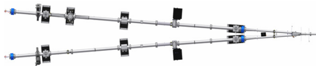
Figure 2: The new IR vacuum chamber layout (half).
