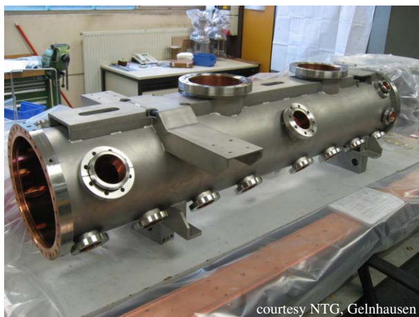
Figure 2: New RFQ-tank upside down with 6 mm wall thickness, reinforcement rail and three point suspension.
