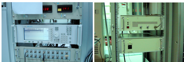
Figure 3: New solid-state RF oscillator and amplifier.
