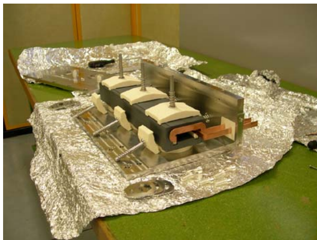
Figure 4: Assembly of the magnet module.
