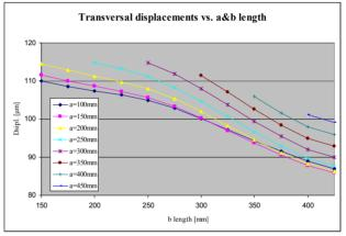
Figure 4 : Transversal frame displ. vs. A and B length.
