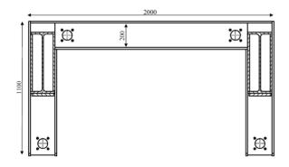
Figure 7 : Undulator frame horizontal cross section.
