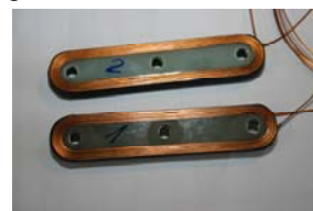
Figure 4: Calibration coils. The coils are made by a 54 filaments NbTi wire. The dimensions of the rectangular wire are 0.46 \times 0.72 \text{ mm} . Each coil has 8 \times 8 layers.
