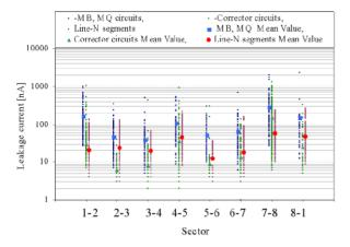
Figure 4: Leakage current versus circuits for all sectors.
