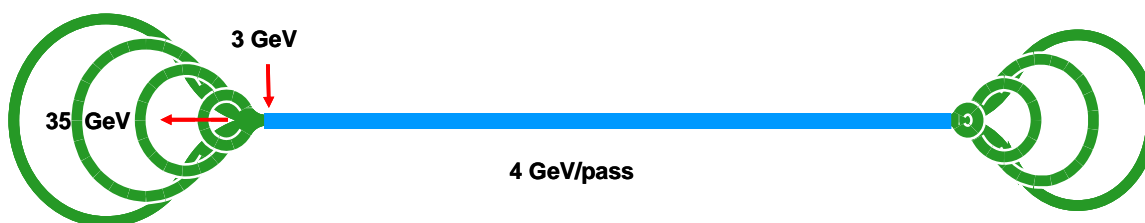
Figure 1: Layout of an 8-pass ‘Dogbone’ RLA with the top-to-injected energy ratio of 12.
