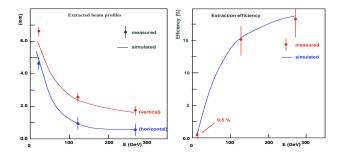
Figure 4: Efficiency and profile widths measured and simulated
