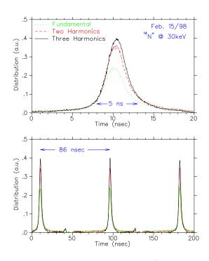
Figure 5: Beam bunches measured on the fast Faraday cup in LEBT for one, two or three harmonic bunching.
