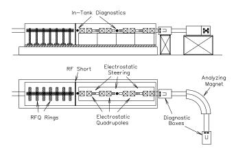
Figure 2: A schematic view of the RFQ and test station.
