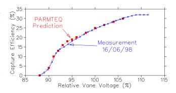
Figure 6: Initial beam test measurement with unbunched  $N^+$  beam. Shown is the measured capture efficiency as a function of vane voltage and the corresponding prediction from PARMTEQ.
