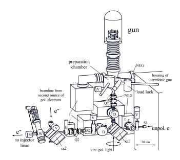
Figure 1: MAMI - source of polarized electrons at the injection point.  $\alpha$ : alphamagnet, D: diff. pumping stage, E: emittance filter, I: ion getter pump, Q: quadrupol, S: solenoid, V: all metal valve, W: wire scanner
