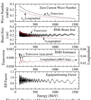
Figure 5. Design and beam simulation results of the superconducting linac section
