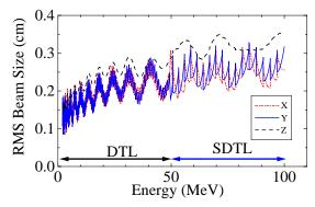
Figure 4. Beam sizes at the DTL and the SDTL
