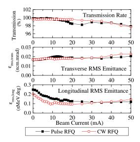
Figure 3. Transmission rate and normalized rms emittance for the pulse mode and the CW mode RFQs
