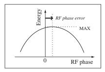
Figure 1: The definition of the RF phase in the SLAC linac.
