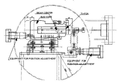
Figure 3: Cross-sectional view of the ESS.
