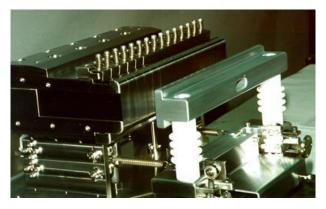
Figure 4: Fabricated electrostatic septum (ESS).
