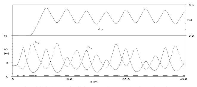
Figure 4: Optical functions for 1/6 of the booster, from center of straight to middle of arc.
