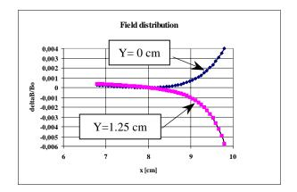
Figure 6: Relative magnetic field distribution for different y-values.
