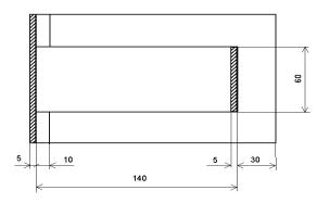
Figure 2: Schematic drawing of the kicker magnet.
