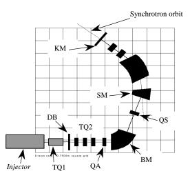
Figure1: General layout of the injection beamline.
