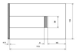
Figure 5: Schematic drawing of the septum magnet.
