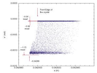
Figure 2: Gold ions distribution in the horizontal phase space at the end of the crystal.
