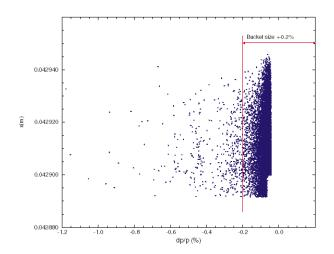
Figure 1: Distribution in x vs. dp/p phase space at the crystal end.
