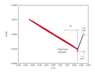
Figure 3: Gold ion distribution in the horizontal phase space at the primary collimator.
