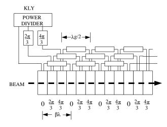
Fig.1 The principle diagram
