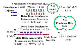
Figure 9: A Two-Beam Accelerator test facility
