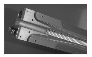
Figure 7: A four-channel decelerator structure.
