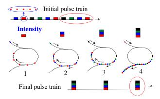
Figure 1: Times-four combination in a ring.
