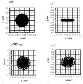
Figure 1. Emittance growth and halo formation of 150 keV, 0.1 A, 0.06  $\pi$  cm mrad proton beam with truncated at 2.6 $\sqrt{\langle x^2 \rangle}$  Gaussian distribution in linear focusing channel.
