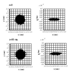
Figure 2. Conservation of 150 keV, 0.5A, 0.07  $\pi$  cm mrad proton beam with distribution, Eq. (22), in nonlinear focusing field, Eq. (27).
