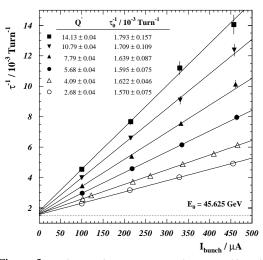
Figure 3: Coherent damping rate as function of bunch current measured at a beam energy of 45.625 GeV for several chromaticities Q'. The straight lines are fits to the individual samples. The table gives measured chromaticities and 'zero current' damping rates.
