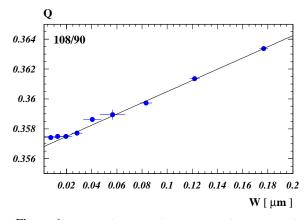
Figure 6: *Tune as function of Courant-Snyder invariant for the data smaple shown in fig. 1 and fig. 5 (the straight line is a fit to the data).*
