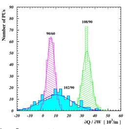
Figure 7: Horizontal detuning with amplitude for the LEP physics optics with horizontal/vertical phase advance in the arcs of 90/60, 102/90 and 108/90 degrees. The distributions of the 102/90 measurements show a larger scatter because of the shorter damping time due to higher beam energy and the resulting fewer data points for a fit.
