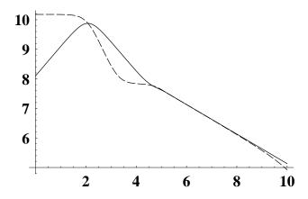
Figure 2: Decimal logarithm of real (full line) and imaginary (dashed line) parts of the transverse impedance in  $\Omega/m$  of the FLHC for the vacuum chamber parameters listed in Tab. 2 on a logarithmic frequency scale from 1 to  $10^{10}$  Hz
