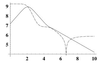
Figure 1: Decimal logarithm of real (full line) and imaginary (dashed line) parts of the transverse impedance in  $\Omega/m$  of the LHC for the vacuum chamber parameters listed in Tab. 2 on a logarithmic frequency scale from 1 to  $10^{10}$  Hz
