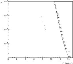
Figure 3: Dynamic aperture D versus number of turns N for the LHC off momentum ( $\delta=1$ ), with modulation ( $\epsilon=2$ ). Tracking data (error bars), interpolation according to Eq. (2) (solid line) and prediction through Lyapunov exponent (squares).
