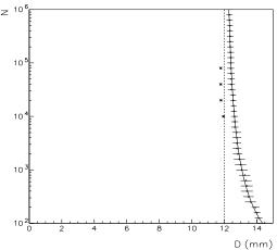
Figure 1: Dynamic aperture D versus number of turns N for the LHC on momentum, without modulation ( $\epsilon = 0$ ). Tracking data (error bars), interpolation according to Eq. (2) (solid line) and extrapolation at infinity (vertical dotted line), prediction through Lyapunov exponent (squares).
