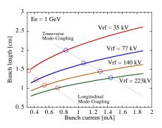
Fig. 2. Bunch lengthening due to potential-well distortion. The mode-coupling starting points are indicated by open circles together with lines for guide the eyes.
