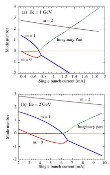
Fig. 1. Eigenvalues as a function of single-bunch current at 1 GeV and 2 GeV.
