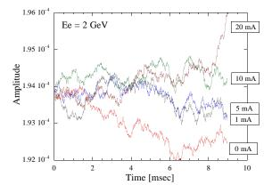
Fig. 3. Amplitude growth as a function of time.
