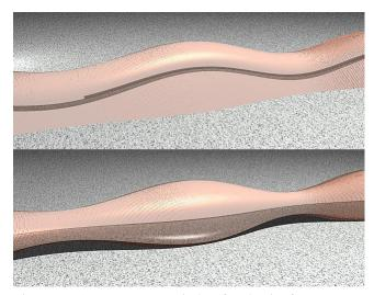
Figure 1: Approx. two periods of pole tip for a vane electrode (top) and a rod electrode (bottom).
