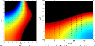
Figure 6: Electric potential and field in cell 114 of Design 4. Left - transverse, Right - longitudinal.
