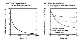
Figure 1: Time Dependence of Beam Current and Vacuum Pressure: these two data was taken simultaneously.
