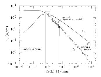
Figure 1:  $R_L$ , when averaged over bins, as given by the FD method (histogram);  $R_L$  and  $X_L$  as given by the CFD method (solid lines) and by Eq. 2 with  $\alpha = 0.5$  (dashes).
