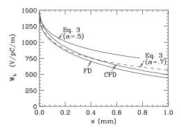
Figure 2: The wakefield of our periodic model, as obtained by different frequency domain methods.
