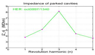
Figure 3: Estimate of  $Z_n$  at first few revolution harmonics, extracted from bunch currents and synchronous phases. Large value at n = 3 is due to the fundamental resonances of parked cavities.
