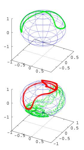
Figure 2: Upper: locus of  $\hat{n}$  for 20  $\pi$  mm mrad vertical emittance. Lower: locus of  $\hat{n}$  for 40  $\pi$  mm mrad and of the anti–damped spin after resonance crossing.
