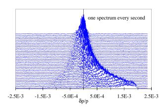
Figure 4: Waterfall diagram of Schottky spectra from stochastic cooling of a Carbon beam. Time proceeds upwards from the bottom.
