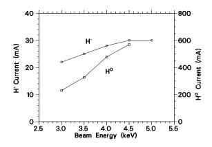
Figure 3:  $H^-$  ion current and  $H^0$  beam intensity within the Na negative-ionizer acceptance versus beam energy.
