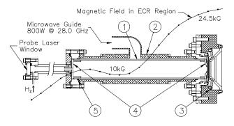
Figure 1: Schematic of ECR proton source; (1) quartz tube; (2) ECR cavity; (3) three plate extraction electrodes; (4) boron nitride end cups; (5) indium seal.
