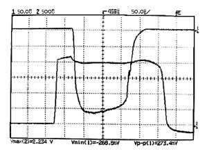
Figure 4: H<sup>-</sup> beam current (negative pulse) and 4.0 kV extraction voltage, 50  $\mu$ s/div.
