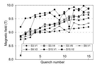
Fig.4 First 15 training quenches of recently tested models
