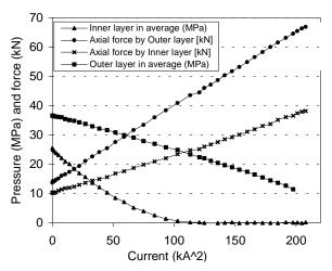
Fig. 3. Coil stress and axial forces of S15.
