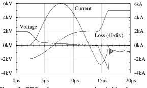
Figure 3. GTO voltage, current, and switching losses.
