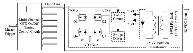
Figure 7. Block diagram of the GTO gate drive.
