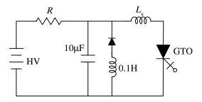
Figure 2. GTO test circuit.
