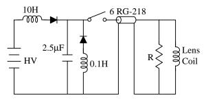
Figure 1. Circuit diagram of the pulser.
