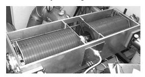
Figure 1: Ferrite loaded cavity C02
