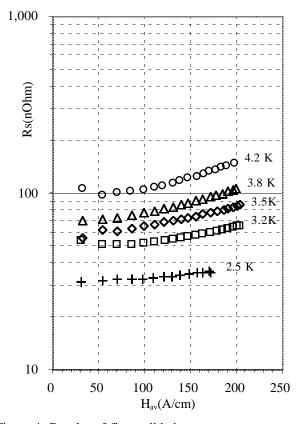
Figure 4: Results of first validation measurements on an Nb test cylinder.
