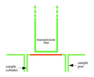
Figure 3: Stripline piece fed by two-wire transmission line. Compared to Fig. 2 the viewing angle is turned by 90°.
