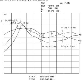
Fig. 3 : Transfer function of the D-coupler for various capacitor gaps.
