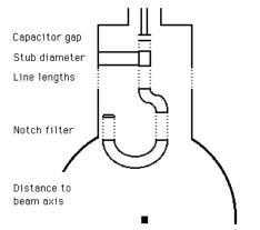
Fig. 2 : Sketch of the variable elements of D-coupler
