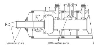
Fig. 1 : Layout of the cryostat with cavities and HOM dampers.
